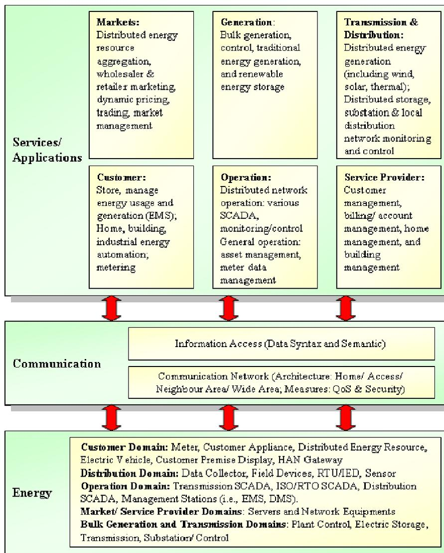
Figure 3. Key elements of a smart grid.
