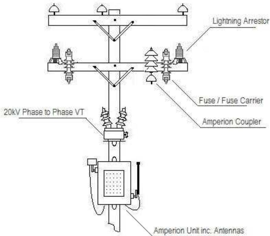
Figure 6.4: Unit installation
