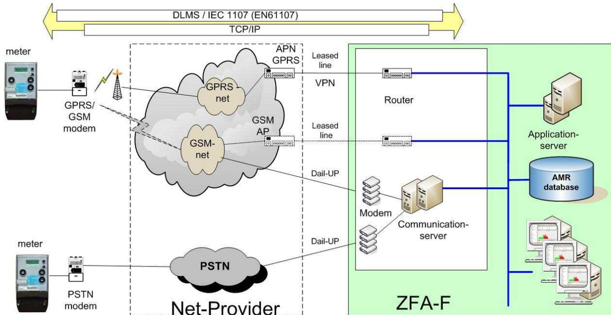
Figure 6.1: The communication system deployed by PPC
