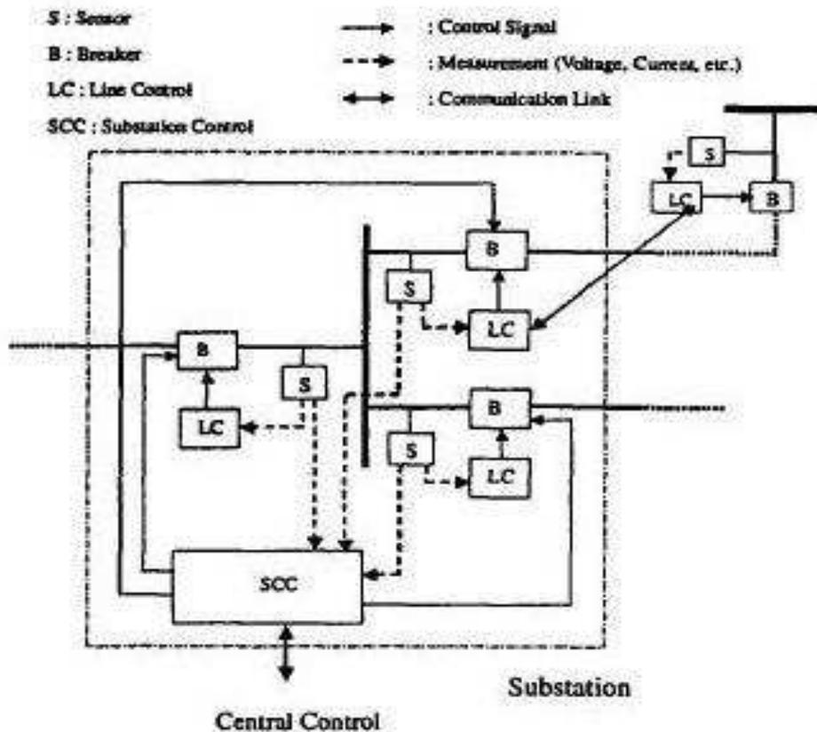
Figure 4.1: Substation coordinated control where a substation controller communicates with line controllers and a central controller to provide flexible protection and control
