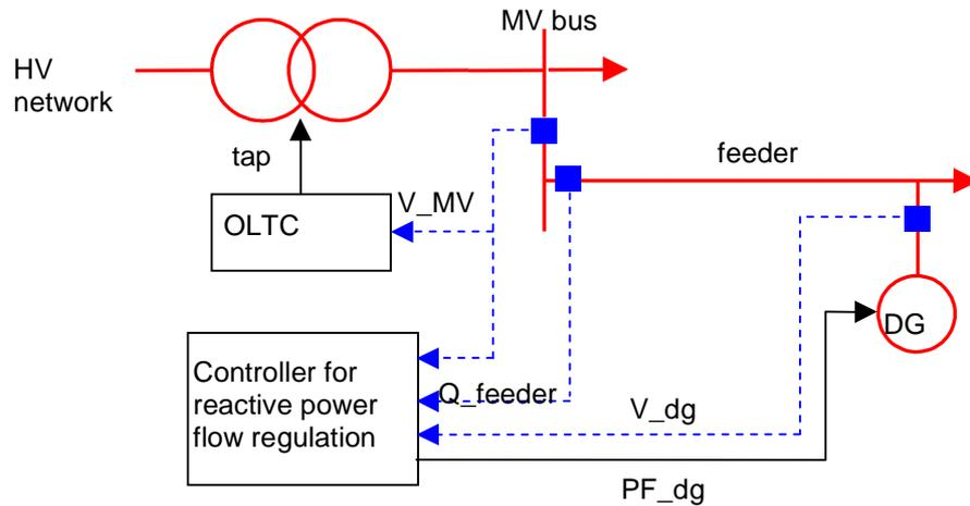
Figure 2.1: Communication architecture for a coordinated control of active distribution network
