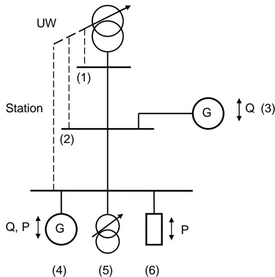
Figure 3.1: Various measures for voltage control
